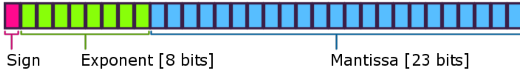
Figure 35: IEEE754 Single-precision floating-point format (Binary32) [8]
