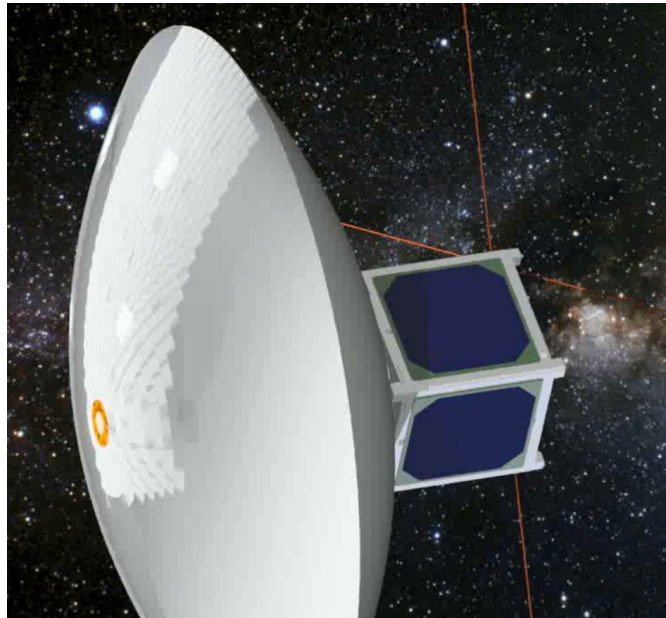
Figure 54: CAD model of inflatable antenna [1]
