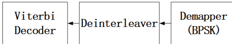
Figure 20: The deinterleaver module also must be compatible with any changes to the data-type made by the mapper for the Viterbi decoder.
