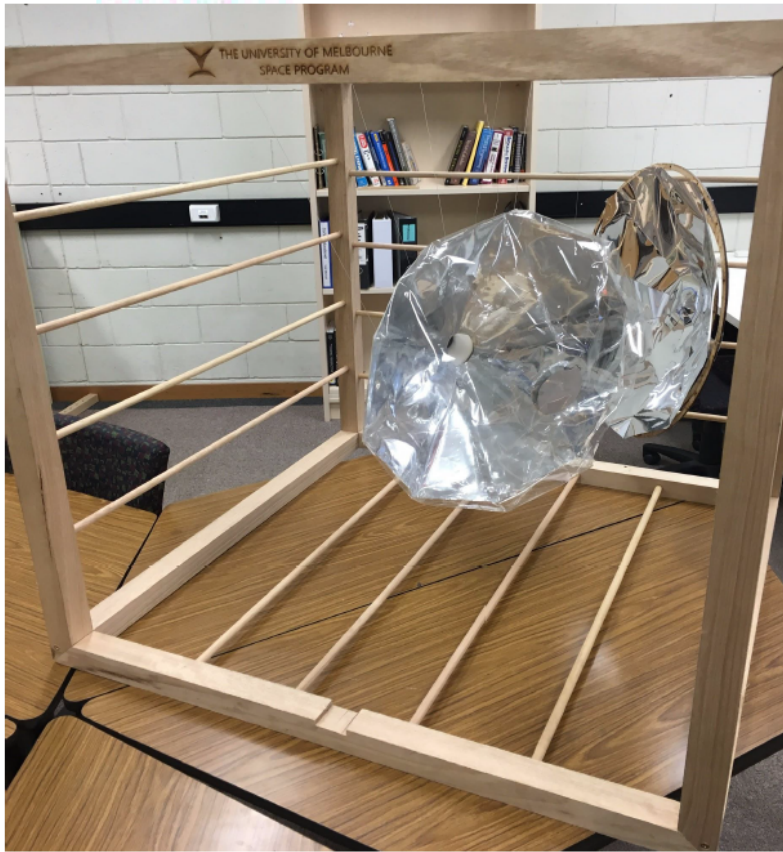
Figure 61: The first inflatable antenna prototype of geometry.
