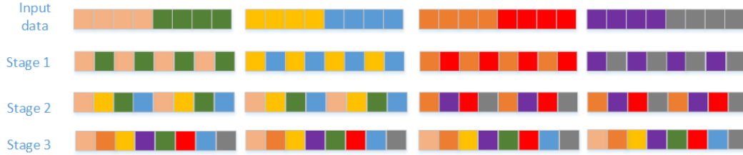
Figure 30: Cycle-efficient interleaving to an arbitrary bit-depth 2^N .
